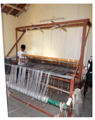
recycling of discarded plastic bags. The discarded plastic bags are washed, cleaned, dried, and cut into strips and woven into the basic plastic textile fabric, which can then be stitched into various products like mats, folders, hand bags and purses. Plastic waste then becomes more manageable and less destructive. The poly loom, which will also start weaving jute, has also provided employment to the local women.
