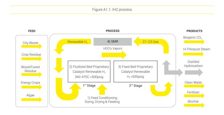
**Applications:** The petrol and diesel produced through this method will conform to Bharat VI norms and can be used directly in cars, trucks, engines etc.
