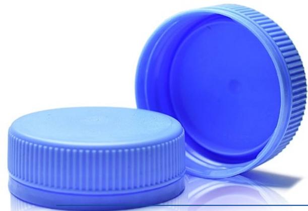
During the recycling process, plastic closures are shredded together with PET bottles. Since polyolefins are less dense (density=0.90 g/cm<sup>3</sup> to 0.96 g/cm<sup>3</sup>) than water (1 g/cm<sup>3</sup>), shredded closures float on the surface and are separated from the more dense PET flakes (1.35 g/cm<sup>3</sup>), which settle at the bottom of the sink-float tank.
