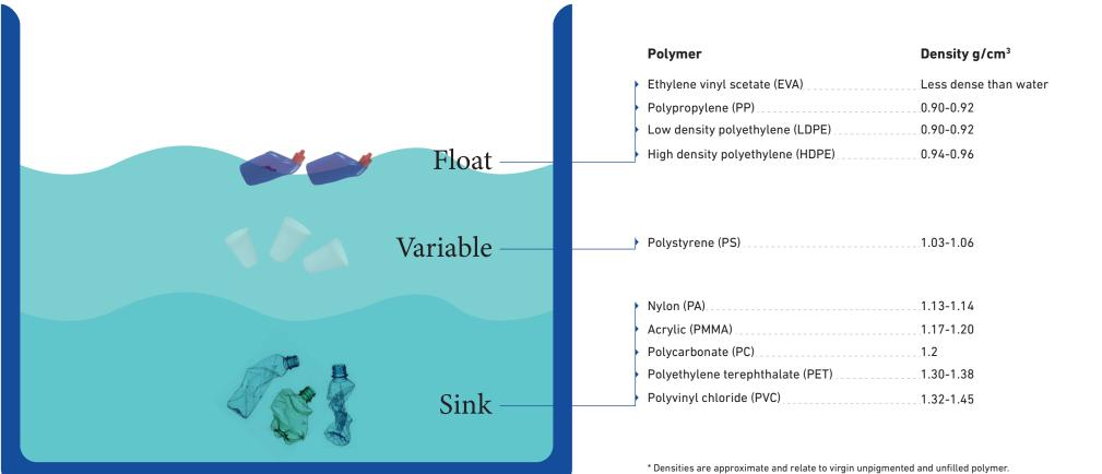
Colouring with a 4% pigment can raise density by 0.03 g/cm<sup>3</sup> which may cause further overlaps of polymer densities.
