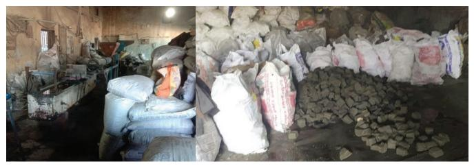
Figure 5: A Type 2 recycling unit manufacturing recycled blocks from mixed plastics
