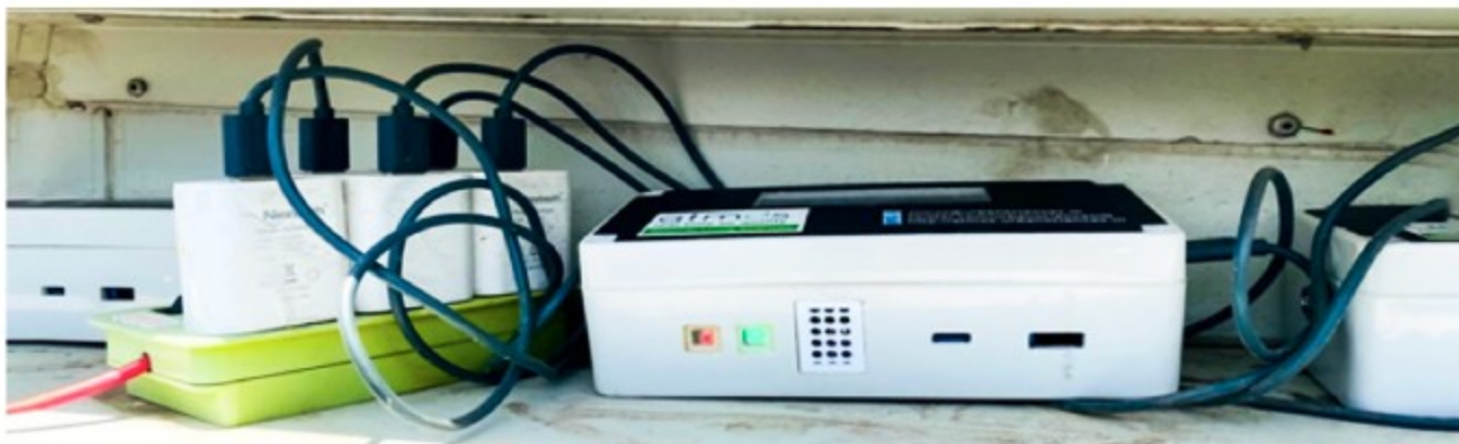
Figure 2.2: Sensor based air quality monitors collocated with the reference-grade air quality monitoring station in Indore.
