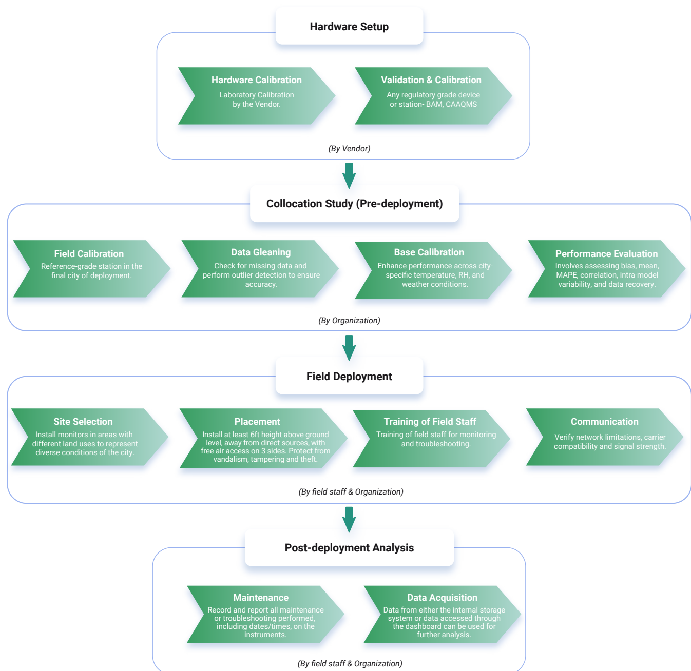
Figure 2.3: Installation protocols for PM 2.5 Air quality Sensor in Field
