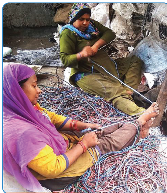
Wire stripping to remove copper from PVC covers in New Seelampur
